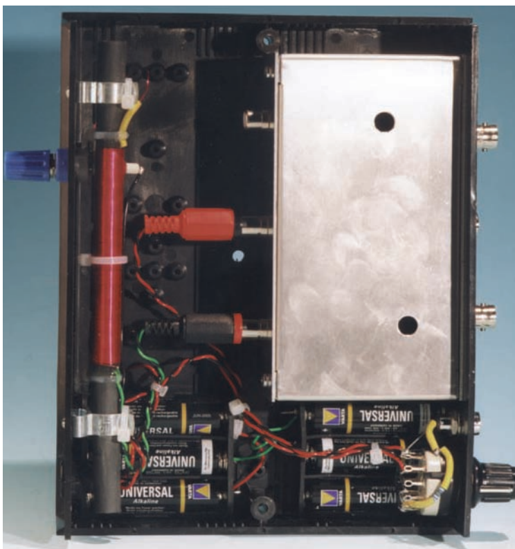
● Fig. 3: It's a good idea to follow this general layout when you come to making your own unit. The blue terminal post is for attaching an external long wire antenna.
