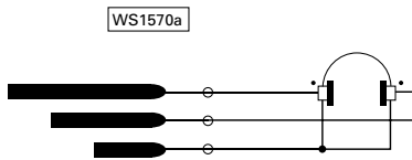
● Fig. 4a: Shows how a pair of stereo headphones which are arranged for normal use in a stereo socket. The dot at one end of each coil represents the same end (be it beginning or end) of each coil winding. The stereo phones are in phase with 8Ω per channel (see text).
